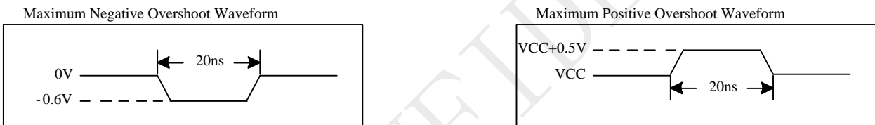
Figure 5-2 Input Test Waveforms and Measurement Level
